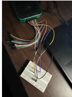
Figure 9. RC low-pass filter on the breadboard.
